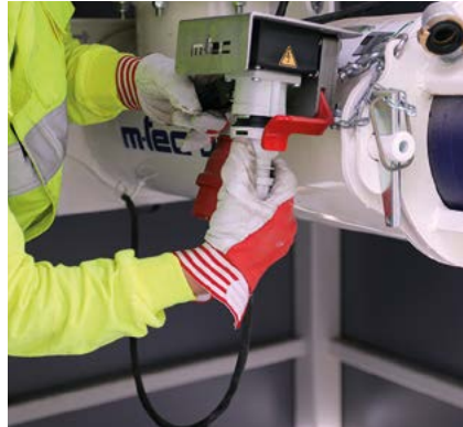
Connect the power cable of the motor of the automatic mixer to the control panel.
